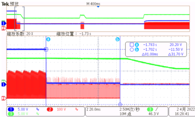
(CH1-Vo, CH2-VDrain, CH3-VDDL) Comments: Protection enter
