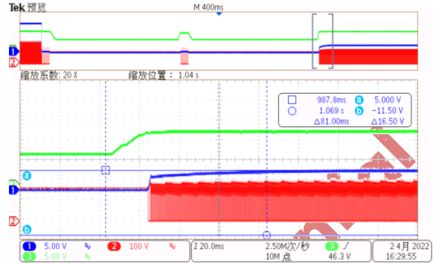
(CH1-Vo, CH2-VDrain, CH3-VDDL) Comments: Recover to 5V
